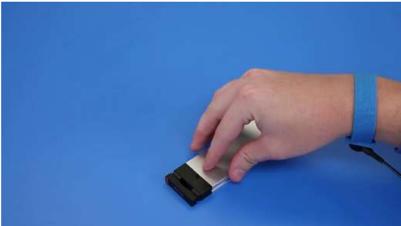
d) Slide the SSD out of the M.2 slot on the carrier.
